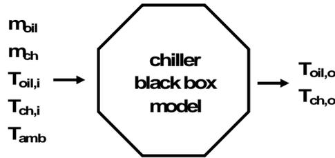
Fig. 6. Absorption chiller black box model.
