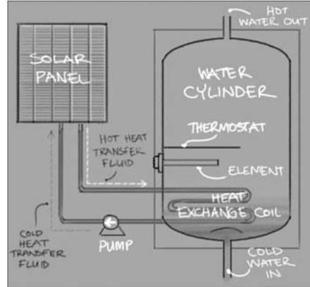
Diagram of a closed loop system
