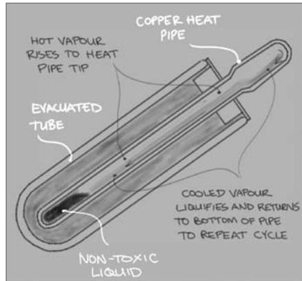
Diagram of an evacuated tube
