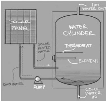
Diagram of an open loop system
