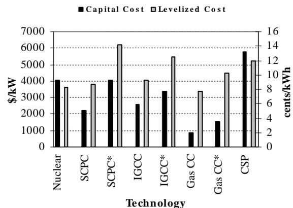
SCPC = supercritical pulverized coal; IGCC = integrated gasification combined cycle; CC = combined cycle; \* = with carbon capture and storage
