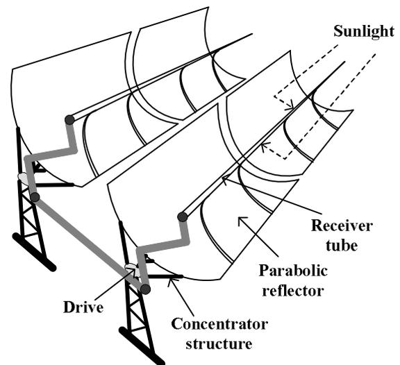
**Fig. 1** Solar collector assembly
