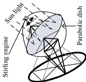
**Fig. 4 Parabolic dish**
