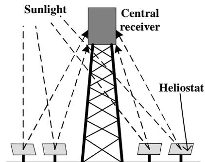
**Fig. 3 Solar Tower or Central Receiver**
