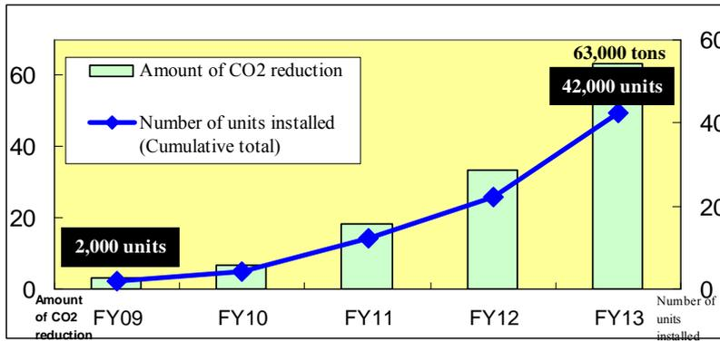
As compared to the conventional systems, "ENE FARM" delivers a CO<sub>2</sub> reduction of 1.5 tons per household per year.\* It equals to 1kg per person per day. (based on Tokyo Gas calculation).
