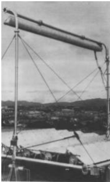
Fig. 1: The linear Fresnel array built by G. Francia in 1963 at Marseilles. It achieved 60% efficiency at 100 atm. and 450°C.
