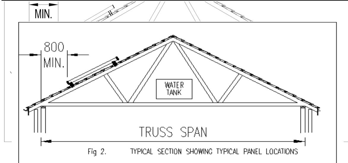
Fig 2. TYPICAL SECTION SHOWING TYPICAL PANEL LOCATIONS
