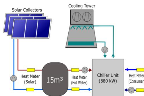
Fig. 7: Simplified hydraulic schema of IKEA.
