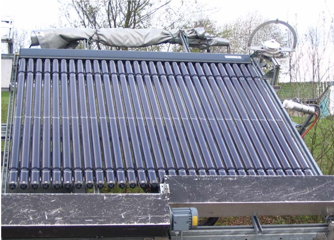
Fig. 4-1: Picture of the collector, mounted in the sun simulator SUSI I
