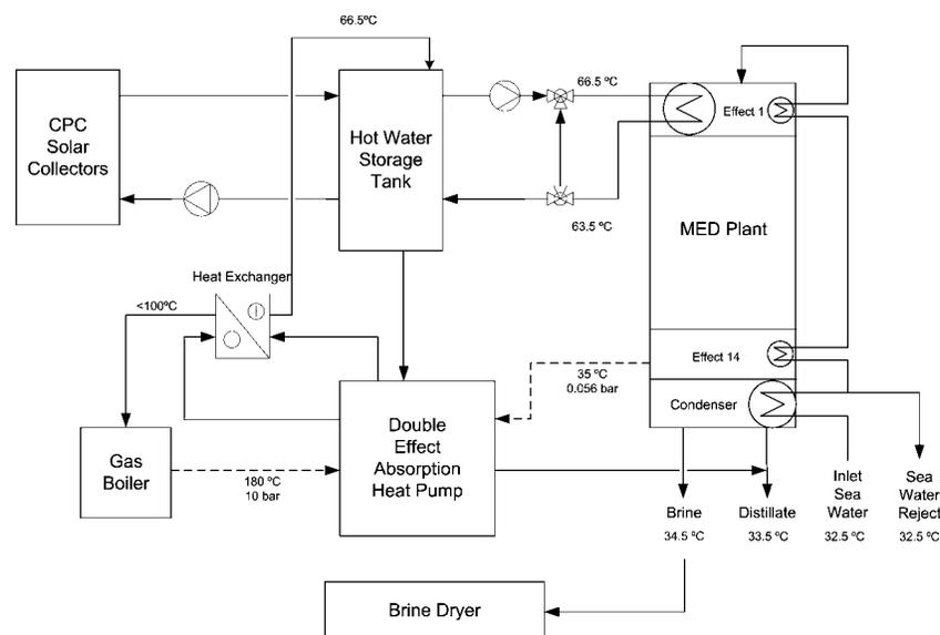
**Figure** Configuration proposed for AQUASOL Plant
