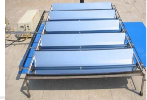
Evacuated glass tube solar air heater
