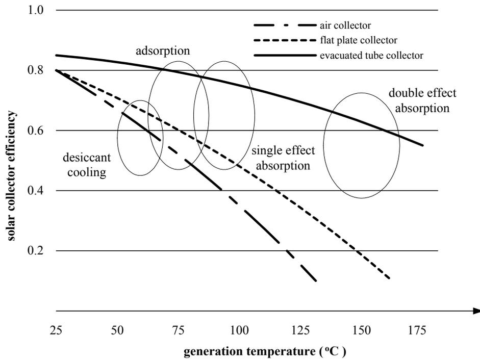
Figure 7. Possible combinations of solar thermal and sorption refrigeration technologies
