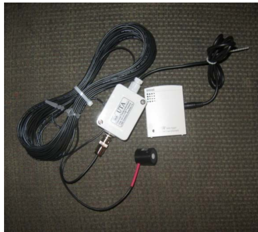
Figure 21: Li-Cor pyranometer connected to amplifier and data logger
