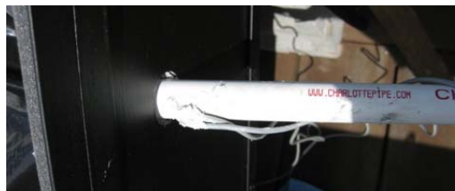
Figure 14: Sensors in inlet and outlet
