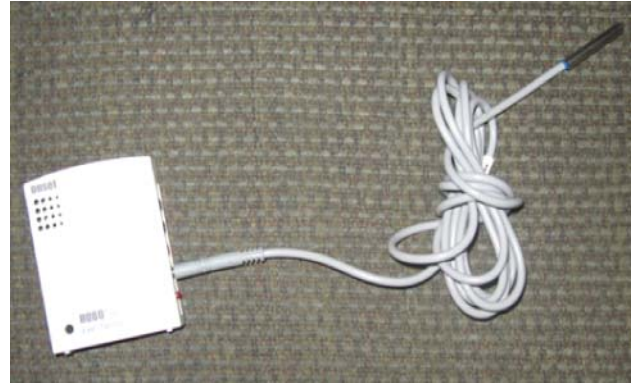
Figure 18: Onset temperature sensor connected to HOBO data logger
